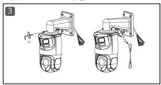
Connect the camera's wiring. Attach 1 and 2 together. Feed 3 through 4/5/6. Insert 3 into 1+2. Secure 4 to 1+2+3. Insert 5 into 1+2+3+4. Screw 6 into 1+2+3+4+5.
